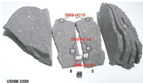
Fig. 1. Smithsonian sample 3509 of the CV3 meteorite Allende sawed into \sim 1 -cm-thick slabs (a centimeter-sized cube marked "T" is included for scale). Refractory inclusions suitable for both thin sectioning and crushing into powders were identified as shown here for slabs 5 and 6. After recording their locations, CAIs were cored out from slabs, and both thin sections and thick butts were produced. Part of the remaining sample was carefully excavated to avoid contamination from matrix materials and crushed into powders for spectral measurements.
